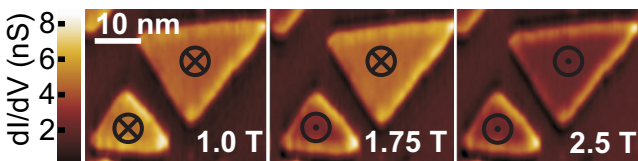
FIG. 2. (Color) Differential conductance images of two Co islands measured at 8 K at 1, 1.75, and 2.5 T with tip ⑤ of Fig. 1 ( U_{\text{gap}} = -0.52 V, I = 1.0 nA). The magnetization of the small island switches between 1 and 1.75 T, and between 1.75 and 2.5 T for the larger island. \otimes indicates a magnetization pointing into the surface, \odot indicates a magnetization pointing out of the surface.
