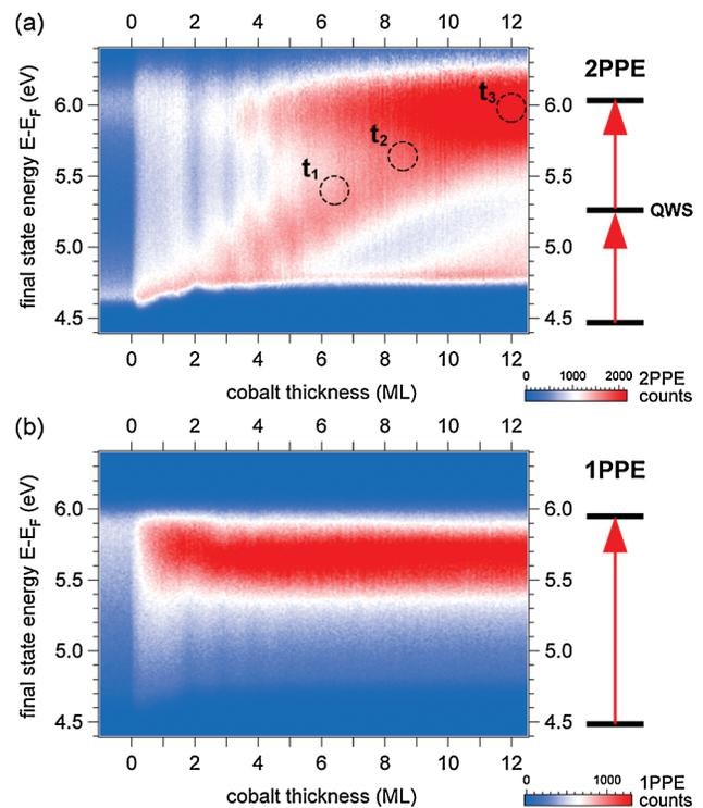
FIG. 1 (color). (a) Thickness dependent 2PPE spectra ( $h\nu = 3.1$  eV) measured in normal emission during the deposition of a Co film on Cu(001). Three selected positions of the quantum well state are marked by  $t_{1,2,3}$  (see text). (b) Equivalent experiment as in (a) but with one-photon photoemission (1PPE,  $h\nu = 6.0$  eV). The excitation light is  $p$  polarized in both cases. General energy level schemes for 2PPE and 1PPE are shown on the side.
