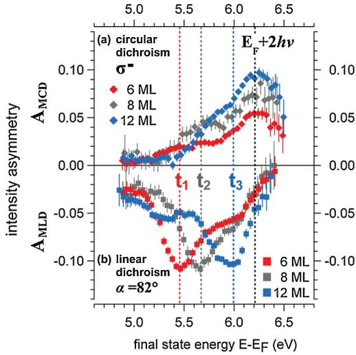
FIG. 3 (color). Thickness dependence of magnetic circular and linear dichroism (MCD and MLD) from Co/Cu(001). MCD obtained with  $\sigma^-$  light and MLD with  $\alpha = 82^\circ$  are shown in the upper and lower panel, respectively. The positions of the QW state  $E_{\text{QW}} + h\nu$  for three different thicknesses are marked by  $t_{1...3}$  (see also Fig. 1). 2PPE from near the Fermi level is indicated at  $E_F + 2h\nu$ .
