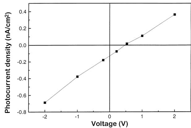
Fig. 5. The voltage dependence of the photocurrent in case of the BiT (thick)/Si heterostructure annealed at  $700^\circ\text{C}$ . The wavelength of the incident light was 350 nm.
