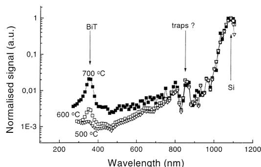
**Fig. 3.** The photoconductive spectral distributions in case of BiT/Si heterostructures with a thick film of BiT (500 nm).
