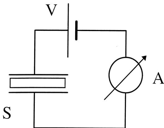
**Fig. 1.** The experimental set-up used for photoconductivity measurements: S, the sample; V, the d.c. voltage source; A, the electrometer.
