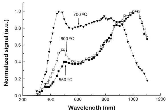
**Fig. 2.** The photoconductive spectral distributions in case of BiT/Si heterostructures with a thin film of BiT (150 nm).
