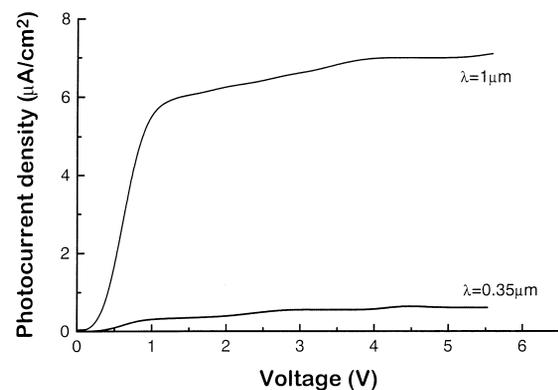
Fig. 6. The voltage dependence of the photocurrent in case of the BiT (thin)/Si heterostructure annealed at  $700^\circ\text{C}$ .
