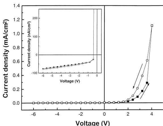
Fig. 4. The I–V characteristic in case of the BiT (thin)/Si heterostructure annealed at  $700^\circ\text{C}$ .
