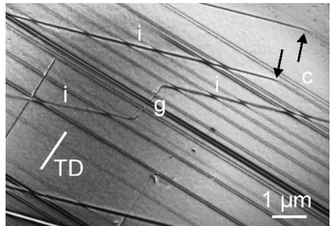
FIG. 5. Micrograph showing traces of periodic dislocations moving on different planes. The inclined planes i may be indexed (0\bar{1}104) and those parallel to the periodic axis g (01\bar{1}00) .
