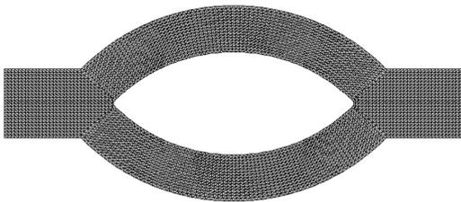
FIG. 2. Finite-element model of a spin-wave interferometer. The curved branches are two  $90^\circ$  segments of a circle with a radius of 170 nm and 36 nm width. The entire structure is approximately 350 nm long. The film thickness is 6 nm. About 42 600 finite elements of tetrahedral shape are used for the simulation. The average volume of the tetrahedral elements is  $(3.26 \text{ nm})^3$ .
