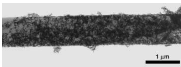
Figure 12. TEM image of a tube with a core-shell morphology, which was prepared by consecutive wetting steps. The outer shell is a network of Pd, the inner core consists of PS.
