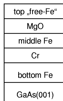
FIG. 1. Schematic view of the complete sample. The magnetization in the middle Fe layer is antiferromagnetically coupled to the bottom Fe layer. The magnetization of the top “free-Fe” layer switches independently.
