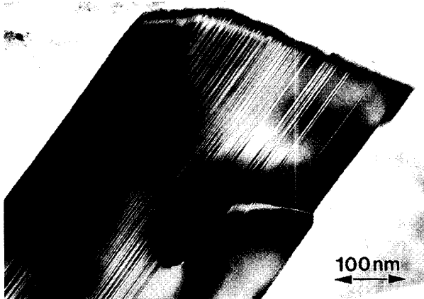
Fig. 3 Cross section TEM image of a Ti-rich grain with a large number of stacking faults on the (001)_{\text{TRP}} planes. Beam direction is [010]_{\text{TRP}} .
