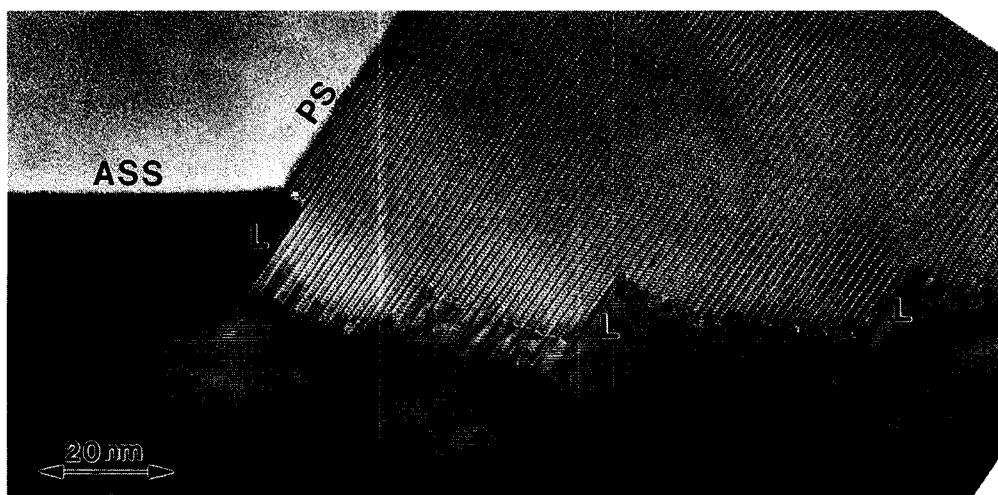
Fig.4 HRTEM cross section image of the reaction front under a Ti-rich grain. Beam direction is [1\bar{1}0]_{BT} = [010]_{TRP} .
