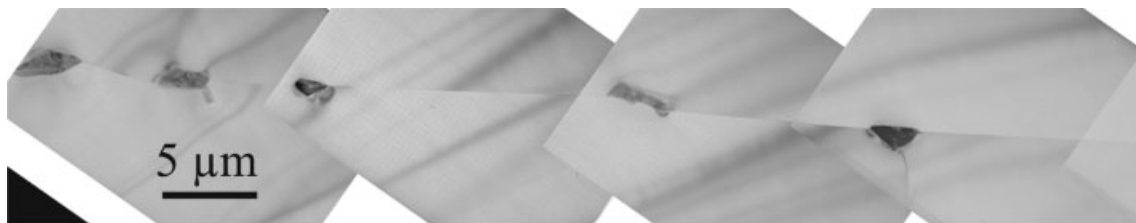
Figure 11. TEM image of SiC precipitates at a large-angle grain boundary inducing an inversion layer
