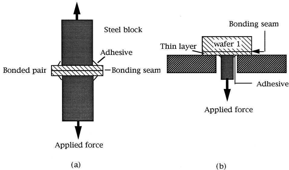
Fig. 3. Schematic of different methods of testing of mechanical properties of bonding interfaces [17].
