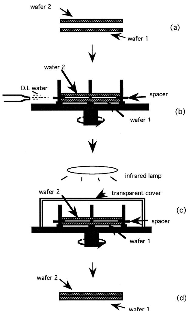
Fig. 1. Schematic of microcleanroom setup and procedure [18].
