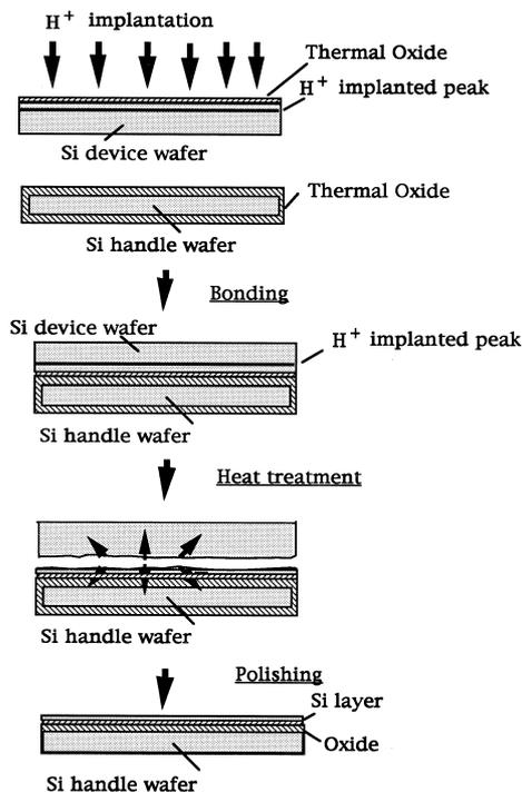
Fig. 10. Schematic of hydrogen-implantation induced layer splitting ('smart-cut') [17,39].
