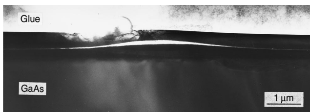
FIG. 10. Cross-sectional TEM picture of hydrogen-implantation induced micro-cracks in GaAs (Ref. 73).
