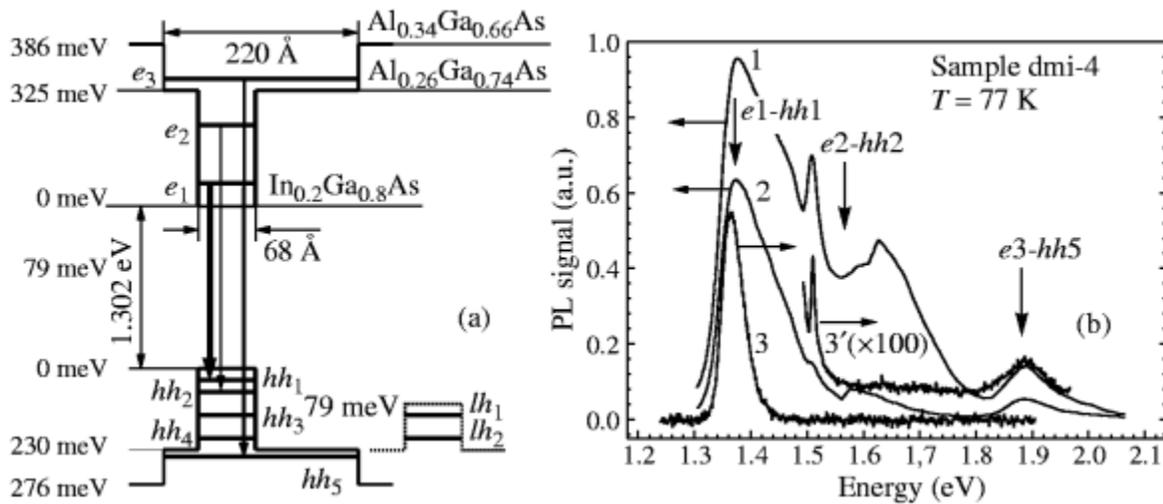
**Fig 3.** (a) Potential profile, subband-edge energies and the main interband electron transitions in QW. (b) PL spectra for different levels of pulse (1 —  $3 \times 10^3$  W/cm<sup>2</sup>, 2 —  $1.8 \times 10^3$  W/cm<sup>2</sup>) and continuous (3, 3' — 20 W/cm<sup>2</sup>) laser pumping.
