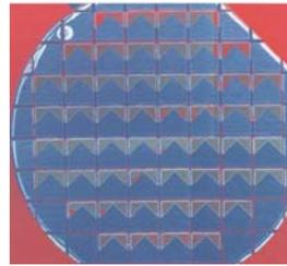
Figure 1: Scanning acoustic micrograph of a bonded wafer pair containing 52 single MC samples
