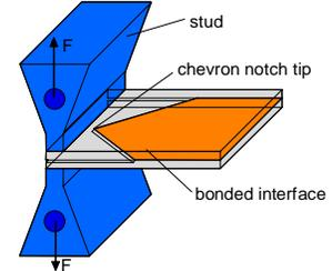
Figure 2: Schematic drawing of the MC-Test arrangement
