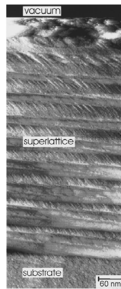
FIG. 3. STM image of a (110)-cleaved 5 \times 10^{18} \text{ cm}^{-3} , Si-doped GaAs/GaAs _{0.7} P _{0.3} superlattice package on a semi-insulating GaAs substrate. The image was taken with a gap voltage of -3 \text{ V} and a tunneling current of 0.5 \text{ nA} .
