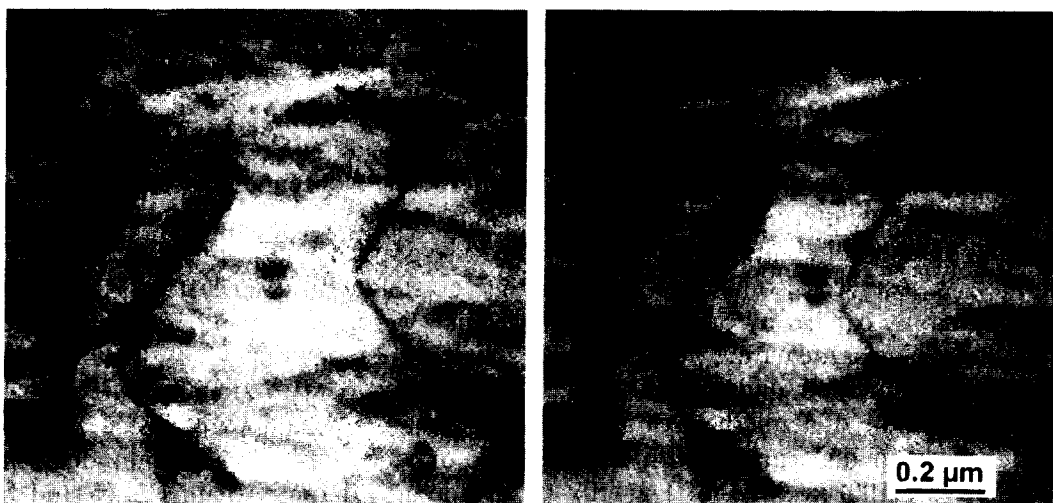
Fig. 1. Two stages of a video record of the viscous motion of a dislocation (marked by arrows) of \langle 100 \rangle Burgers vector on a \{001\} plane during in situ deformation of an NiAl single crystal at 475°C.
