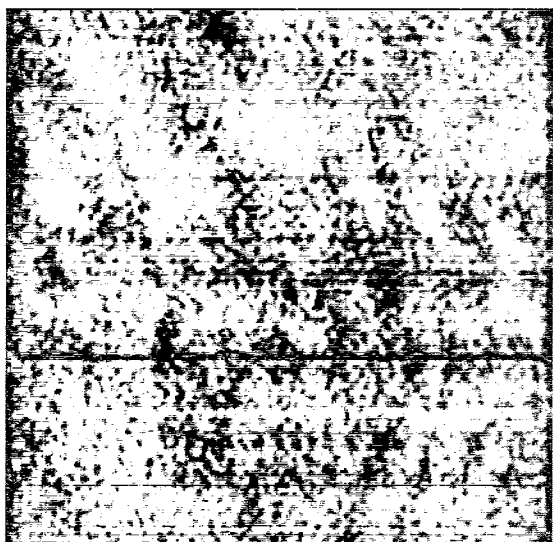
Fig. 1. SEMPA image ( 10 \times 10 \mu\text{m}^2 ) of an as-grown Co film with 3.0 to 3.1 ML thickness. Only the perpendicular component is shown, the in-plane signal vanishes.
