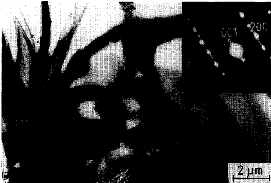
Fig. 13. Transmission electron microstructure taken during in situ pseudoelastic deformation in the \langle 110 \rangle direction of the foil in the [001] zone axis orientation. SADP from the martensite is inserted in the corner of the micrograph.
