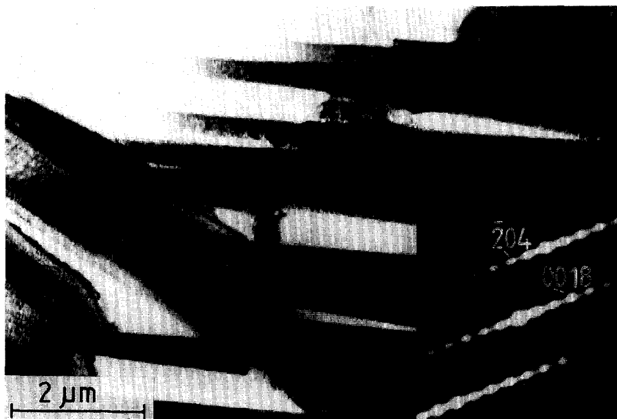
Fig. 9. (a) Transmission electron micrograph showing propagation \beta_1' martensitic needles. SADP is inserted in the corner.
