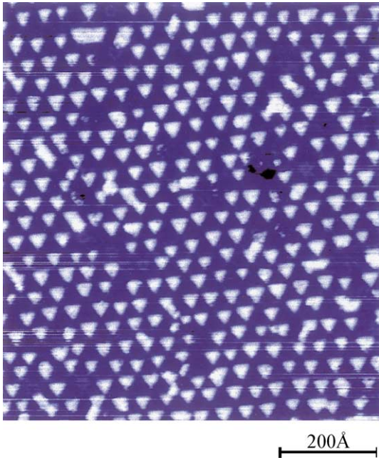
Fig. 6. STM image of a periodic array of Fe islands nucleated on the dislocation network of a Cu bilayer on Pt(1 1 1) at 250 K (image copied from Ref. [22]).
