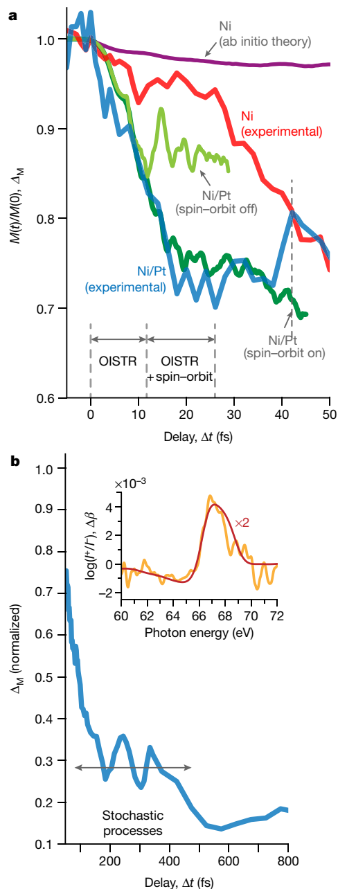
Fig. 3 | Optically induced spin-transfer, post-excitation spin dynamics and quantum dynamical modelling. a , Comparison between the experimentally recorded attosecond MCD trace in Ni/Pt-multilayers (blue line) and pure Ni (red) with the ab initio simulation of light-field-induced spin dynamics, including spin-orbit coupling in the multilayer (dark-green line) reveals that for the first 10 fs the demagnetization of Ni layers is entirely due to flow of majority-spin current across the material interface. Theoretical calculations without the spin-orbit interaction predict saturation of the demagnetization 15 fs after the optical excitation (light-green line). This is a clear indication that beyond this time all the demagnetization is caused by spin flips, whereas at earlier times spin dynamics is governed by OISTR, which is absent in the theoretical prediction for bulk nickel (violet line; see Fig. 2). b , Experimental data recorded for longer timescales in the multilayer system (blue line) indicate complete quenching of the magnetic moment due to stochastic processes with a characteristic timescale of 112 fs. The recorded \Delta_M exhibits additional modulations up to 300 fs after the optical excitation, whose origin remains speculative, but could be rooted in coherent phonon modes affecting the coupling to the lattice. The inset compares the recorded MCD signal \Delta = \log(I^+/I^-) of the Ni/Pt sandwich (orange line) with the imaginary part of the computed magneto-optical function \Delta\beta (red line).
