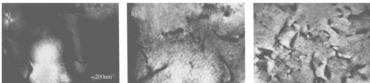
Fig. 2. Dislocation structures in icosahedral Al–Pd–Mn deformed by 0.1 (a), 0.3 (b), and 1.5% plastic strain (c).
