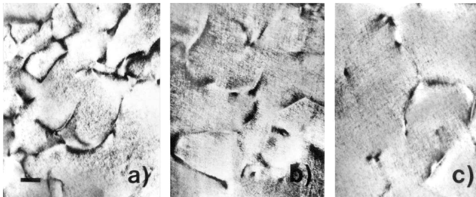
Figure 3. Bright-field electron micrograph of the sample deformed by \varepsilon_{\text{plast}} = 5.2\% ; (a) as deformed; (b) after heat treatment for 13 min at 730^{\circ}\text{C} ; (c) after heat treatment for 90 min at 730^{\circ}\text{C} .
