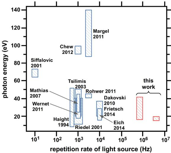
**Fig. 1.** Overview of HHG-based PES setups highlighted by their photon energy range and repetition rate [7–18]. For clarity, the overlapping kHz [9–12] as well as 10 kHz experiments are shown with different width [16–18].
