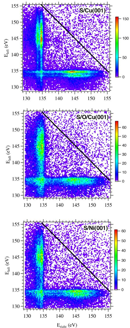
**Fig. 5.** 2D-energy spectra of different samples taken with  $h\nu = 301$  eV photons, (a) S/Cu(001), (b) S/O/Cu(001) and (c) S/Ni/Cu(001). The solid diagonal line marks the energy position of  $E_{sum}^{max}$ .
