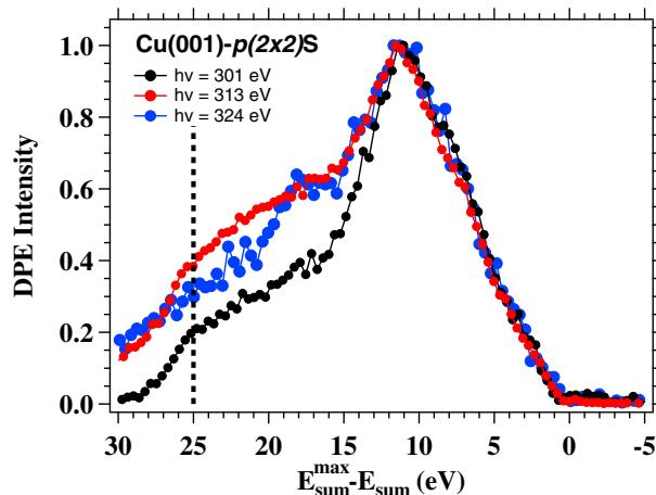
**Fig. 4.** Sum energy spectra obtained from the experiments with  $h\nu = 301, 313$  and  $324$  eV. The dashed vertical line is the energy position of the blue diagonal line of Fig. 3 which is at  $E_{sum}^{max} - E_{sum} = 25$  eV. For better comparison we normalized the spectra such that the maximum intensity is unity. (For interpretation of the references to color in this figure legend, the reader is referred to the web version of this article.)
