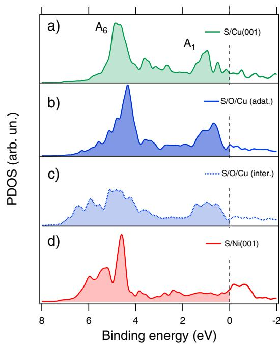
**Fig. 6.** DFT single-particle density of states projected onto the 3p orbitals of the sulfur atom for (a) S/Cu(001), (b) and (c) S/O/Cu(001) and (d) S/Ni(001). The DOS for S/O/Cu(001) has been calculated separately for adatoms (b) and interstitial atoms (c). The dashed line marks the energy position of the Fermi level.
