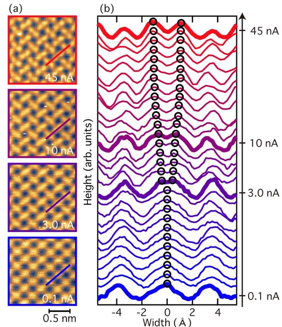
FIG. 2. Current dependence of STM images. (a) Topographic images taken at  $V_s = 0.25$  V with varying  $I$  from 0.1, 3.0, 10 to 45 nA. (b) Line profiles at  $V_s = 0.25$  V, measured along lines indicated in (a). From the top to the bottom,  $I$  varies as follows: 45, 40, 35, 30, 25, 22, 20, 18, 15, 12, 11, 10, 9.0, 8.0, 7.0, 5.0, 3.0, 2.0, 1.0, 0.9, 0.8, 0.7, 0.6, 0.5, 0.4, 0.3, 0.2, and 0.1 nA, respectively. Empty circles indicate peak positions extracted from one Fe dimer.
