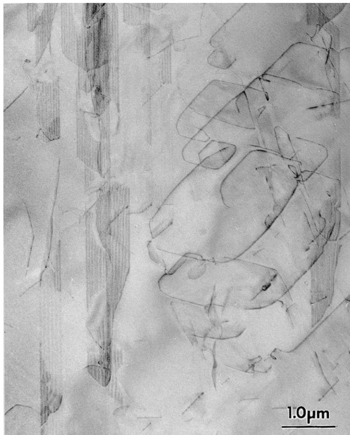
Fig. 1. Dislocation structure after deformation at 610°C. Strain rate 10^{-6} \text{ s}^{-1} , plastic strain 0.6%, twofold compression axis, pseudo-twofold beam direction.
