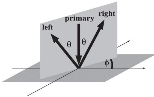
FIG. 6. Sketch of the geometry assumed by (e,2e) calculations from a Cu(111) surface.<sup>26,27</sup> A normal incidence primary electron impinges onto the sample. This is followed by the emission of two electrons with equal energy and equal emission direction with respect to the surface normal. This is characterized by the angle  $\theta$  while the plane containing the primary beam and the outgoing electrons has an azimuthal orientation given by  $\phi$ .
