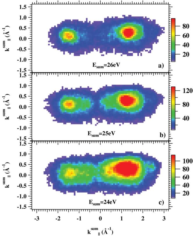
FIG. 4. (Color) 2D  $k_{\parallel}^{\text{sum}}$  distribution for different values of the sum energy. The primary energy was 31 eV. The horizontal axis is along the  $[\bar{2}11]$  direction, which is parallel to the shortest reciprocal lattice vector. The color code for the intensity (in counts) is displayed on the right of each plot.
