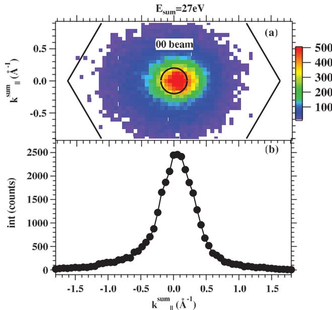
FIG. 9. (Color) In (a), we display the 2D  $k_{\parallel}^{\text{sum}}$  distribution for states near  $E_{\text{sum}}^{\text{max}}$ . The primary energy was 32 eV. We identify the intensity peak as the 00-beam, the circle around this peak marks the momentum range we considered for the momentum plots to be shown below. The black lines indicate the Brillouin zone boundary. In (b), we show a line scan through the intensity peak.
