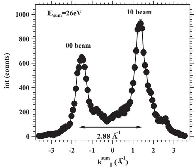
FIG. 5. Line scan along the  $[\bar{2}11]$  direction through the intensity peaks of Fig. 2(a). The sum energy is 26 eV and the labeling of the spots follows the notation used in LEED, see also Fig. 2.
