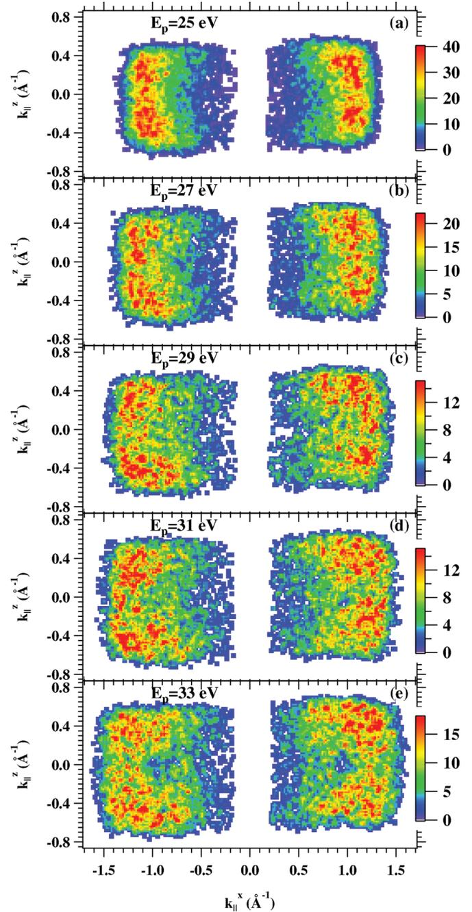
FIG. 13. (Color) These momentum plots are equivalent to Fig. 12 except that the sum energy is 2.5 eV below  $E_{\text{sum}}^{\text{max}}$ . This means that the ellipse defining the energy constraint is now centered at the upper dashed diagonal line in Fig. 7. With this selection we focus on the pair emission from the  $3d$  states.
