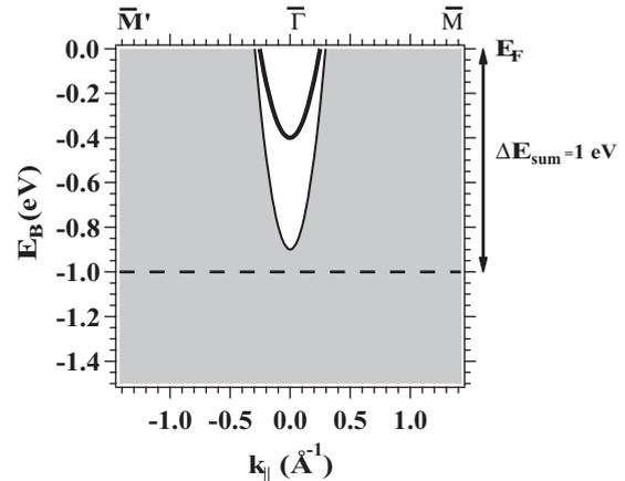
FIG. 3. Simplified band structure of Cu projected onto the (111) surface. The solid line shows the dispersion of the Shockley surface state, which exists in the bulk band gap (white area). The gray area indicates available bulk states. The dashed line marks the available valence states for  $E_{\text{sum}} = 1$  eV below  $E_F$ . The arrow on the right represents the energy resolution of the experiment.
