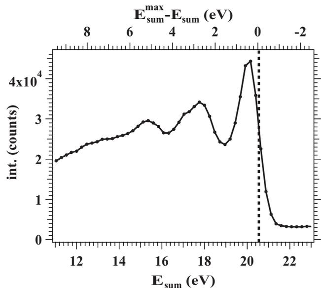
FIG. 8. Intensity vs  $E_{\text{sum}}$  spectrum obtained from the 2D energy distribution presented in Fig. 7. For an easier identification of the energetic position of the valence electron, we use  $E_{\text{sum}}^{\text{max}} - E_{\text{sum}}$  as upper  $x$  axis. The position of  $E_F$  is indicated by the vertical dashed line.
