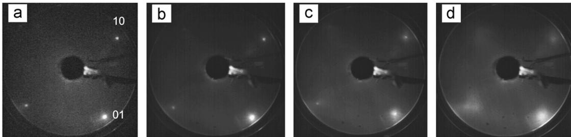
**Fig. 1.** LEED patterns of Fe films on Rh (001) surfaces. The thicknesses are (a) 1 ML, (b) 3 ML, (c) 4 ML and (d) 6 ML. The patterns were taken at room temperature for the electron energy of 37 eV.
