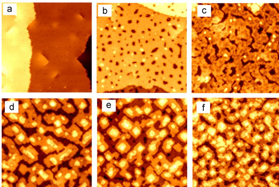
**Fig. 2.** STM images of bare Rh (001) surface (a) and Fe films of different thicknesses (b–f). The thicknesses are (b) 0.9 ML, (c) 1.9 ML, (d) 2.9 ML, (e) 3.9 ML and (f) 5.5 ML. The scan area for all images is  $50 \times 50$  nm. All images were obtained with a W tip.
