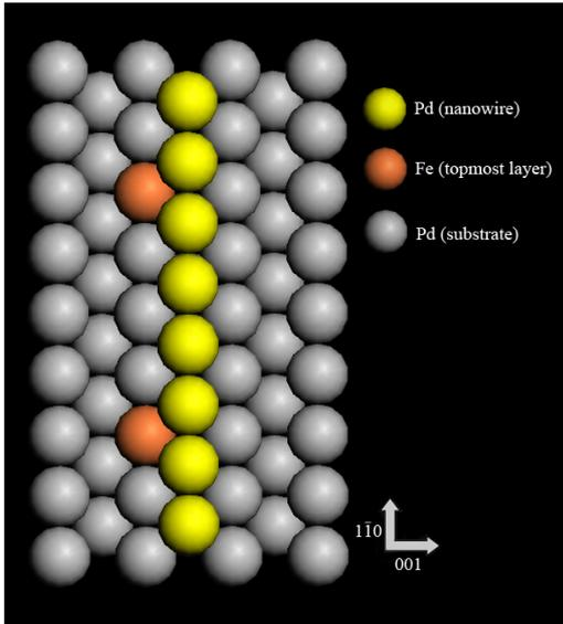
**Figure 1.**  $1.3 \times 10 \times 7$  Pd(110) elementary cell structure (top view).
