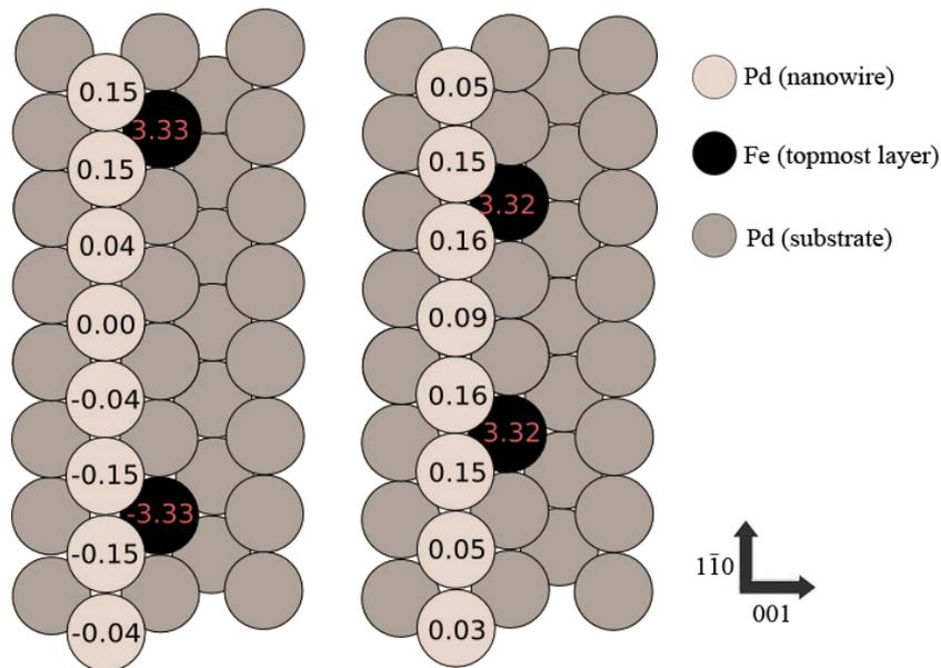
**Figure 4.** Magnetic moments ( $\mu_B$ ) of Pd nanowires grown atop embedded Fe atoms. The left (right) sketch illustrates the case of antiferromagnetically (ferromagnetically) coupled Fe impurities. In the case of antiferromagnetically coupled Fe impurities, the magnetic moments change their sign at the center of the Pd ad-chain.
