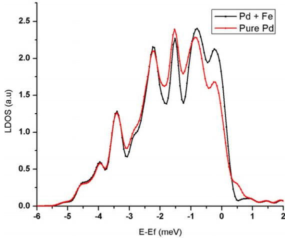
**Figure 3.** Surface chain Pd d-state density. The red graph corresponds to a configuration with a pure Pd surface under the chain, the black one describes chain Pd d-states when one Fe atom is embedded in the topmost layer under the chain. Zero energy corresponds to the Fermi energy.
