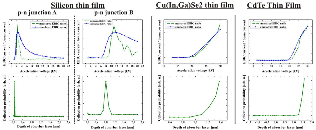
Figure 1: (upper line) Electron energy-dependent EBIC gain of measured (green line) and fitted (blue line) values. (lower line) Collection probability versus depth of the absorber layer derived from the fitted EBIC gain above.
