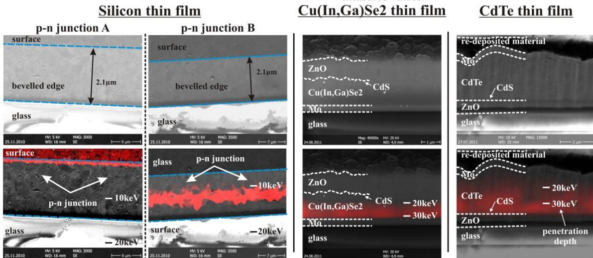
Figure 2: (upper line) SE images of the cross sections of the different thin film technologies. The different layers are enclosed by dotted lines. Note, the Si samples are bevelled cross sections. (lower line) SE images overlaid by EBIC measurements. The p-n junctions are clearly visible as regions with high EBIC signal (red colour).
