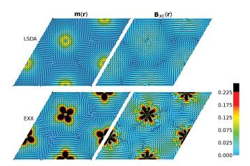
FIG. 1 (color). Fully noncollinear magnetization density and **B** field obtained using the LSDA and exchange-only EXX functionals for an unsupported Cr monolayer in Néel state. Arrows indicate the direction, and information about the magnitude (in atomic units) is given in the color bar.
