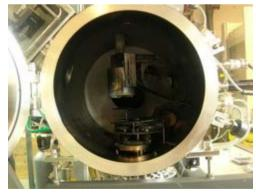
This chamber is used by scientists at the Max Planck Institute for Microstructure Physics to produce the ferroelectric material PZT using pulsed laser deposition (PLD). The method permits extremely accurate control of the material formation.
