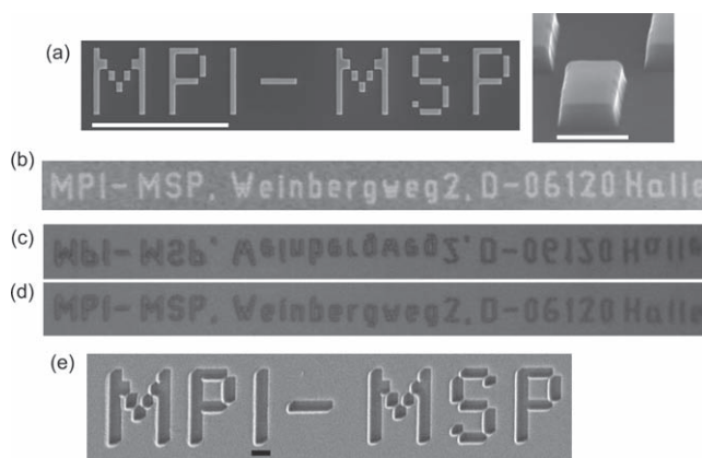
Figure 7. Replication of complex structures. a) SEM and b) optical micrograph (50 \times ) of the master nanopattern showing ca. 400 nm width columns. c) Optical micrograph of the polymer replica with microchannels in a mirror image of the master. d) Flipped image of the replica presented for clarity. e) Corresponding SEM image of the replica. Scale bars: a) 10 \mu\text{m} (left) and 500 nm (right); e) 1 \mu\text{m} .
