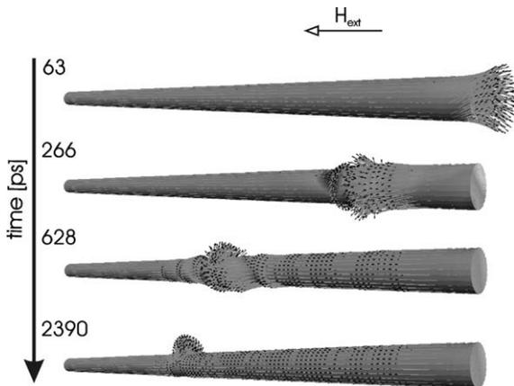
Fig. 4. Dynamic mode conversion in a cone-shaped wire of  $1\ \mu\text{m}$  length and linearly varying diameter between 30 and 60 nm. The reversal starts at the thicker end as a vortex mode. The reversal front propagates along the wire. When it passes through a range of critical thickness, the vortex mode converts into the corkscrew mode.
