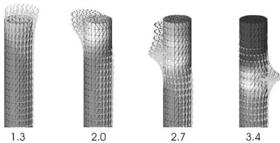
Fig. 1. Snapshots of the initial stages of the “corkscrew” reversal mode in a Ni wire with a diameter of 40 nm; the numbers indicate time in nanoseconds. The wire is exposed to a reversed field of 200 mT. A head-to-head domain wall is nucleated at the end of the wire. It propagates along the wire axis on a characteristic spiralling orbit.
