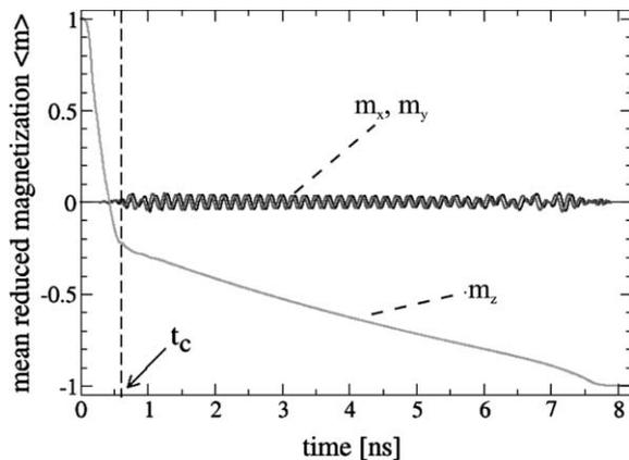
Fig. 5. Average magnetization components during the reversal of the cone-shaped particle. The mode conversion sets in at the time  $t_c$ . At that point, the slope of  $m_z$  changes drastically, indicating the conversion of the fast vortex reversal mode into the slow corkscrew mode. The conversion into the corkscrew mode also reflects in the onset of the characteristic oscillations in the  $m_x$  and  $m_y$  components.
