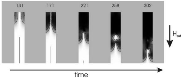
Fig. 6. Formation of magnetic “drops” during the localized curling reversal mode. The images represent the magnetization component parallel to the wire axis (white: up; black: down) on a cutplane through the middle of the wire. The numbers indicate the time elapsed (in ps) after application of the reversed field. Different mobilities of the vortex core and the domain wall on the shell lead to a dynamic equilibrium with periodic disruptions in the reversal front.
