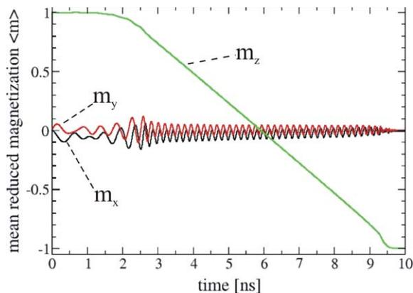
Fig. 2. Spatially averaged magnetization components as a function of time in the case of the corkscrew reversal mode in a Ni nanowire of 40 nm thickness and 1  $\mu\text{m}$  length. The change in the axial magnetization component  $m_z$  indicates the propagation of the domain wall. The gyrating motion of the domain wall around the axis reflects in the oscillations of the perpendicular components  $m_x$ ,  $m_y$ .
