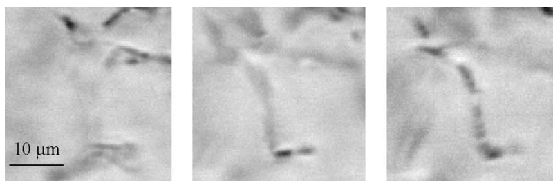
Fig. 4. Scanning infrared images of the same dislocation with the beam focused at different depths in the wafer along the beam direction. The distance between the different positions of the focus is about 50 μm. The sharpest contrast (right image) occurs when the dislocation lies in the focal plane.
