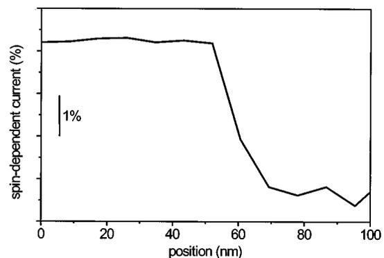
FIG. 4. Line scan across a domain wall between two domains of opposite contrast on Co(0001). The displayed data is raw data of a single scan and was recorded in  $\approx 100$  ms.
