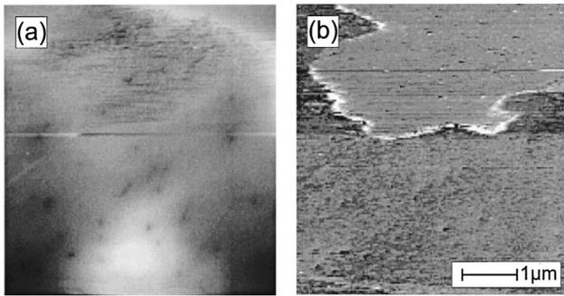
FIG. 1. STM images of the topography (a) the magnetic domain structure of the same area (b) of polycrystalline Ni. Sample bias: 0.13 V; tunneling current: 1 nA; (a) height variations 3 nm; (b) spin contrast: 2.2%.
